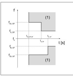
IL "Inner limit" - inner limit valueOL "Outer limit" - outer limit value(1) Trip range
