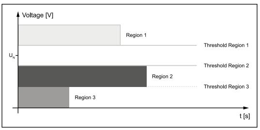
Division of the grid voltage range into three fault regions by selecting the detection thresholds.
