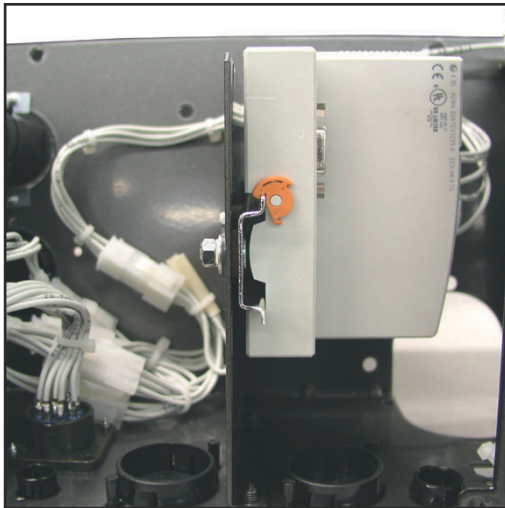
Field bus coupler in interface fitted to insulated DIN rail - TS/TPS, MW/TT series
